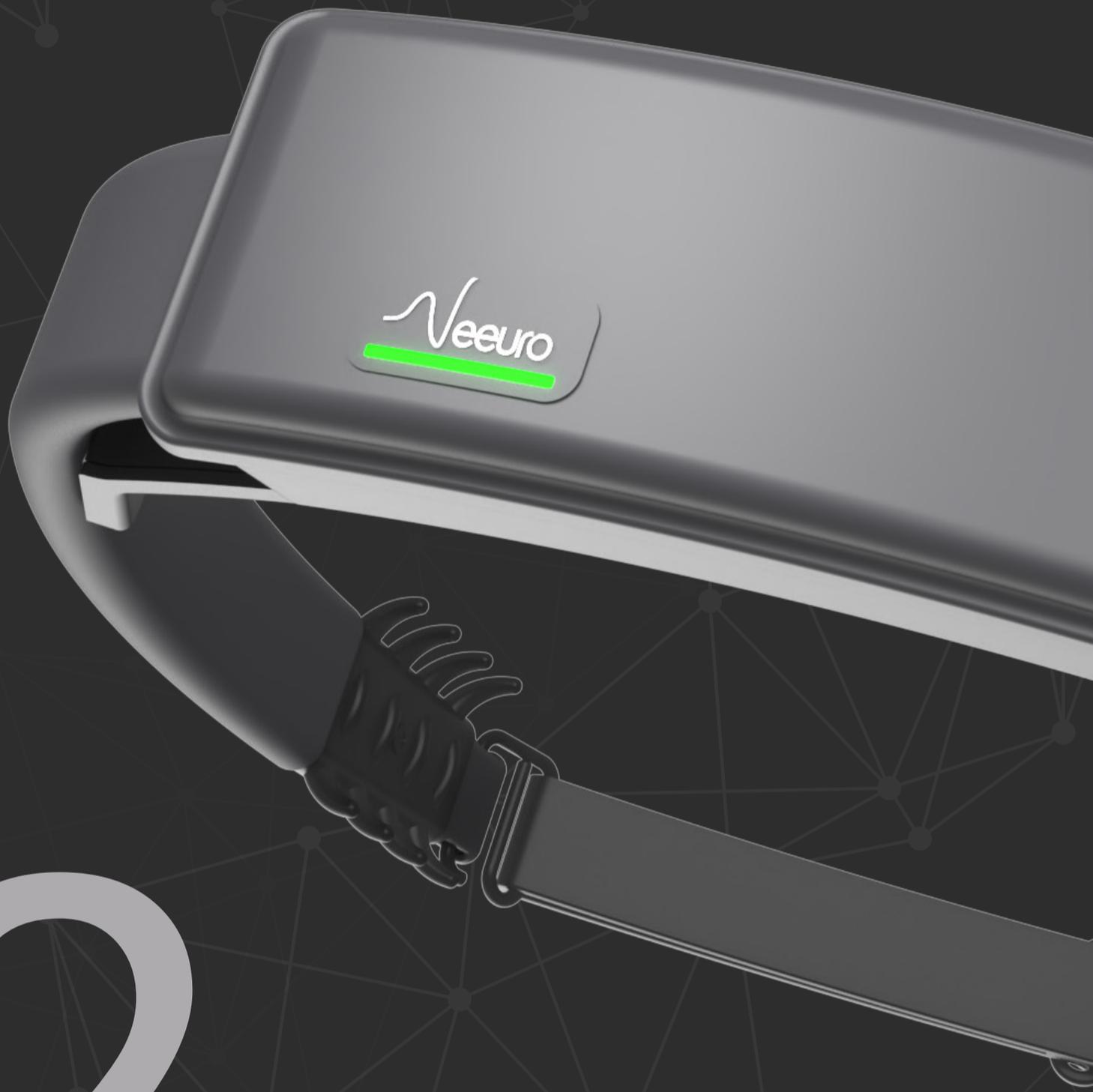
The Neeuro SenzeBand 2 is a non-invasive device for capturing EEG (brainwaves) signals. It consists of 7 dry electrodes with five located on the prefrontal cortex and two on the sides. Together with Neeuro's machine learning algorithms, it interprets various mental states like attention, relaxation, mental workload, fatigue, stress and many more; providing insightful biofeedback for measurements used in real-time to drive interventions for various brain challenges.
